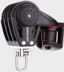
BB-0412FE Triple Angle Cleat Max Lina: 10mm SWL : 320 kgs MAX: 1200 kgs Waga: 172 g
