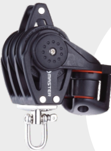
BB-0413FE Triple Bucket Angle Cleat Max Lina: 10mm SWL : 320 kgs MAX: 1200 kgs Waga: 175 g
