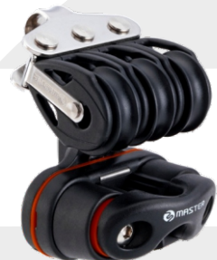
BB-2212F Triple Bucket Cleat Lina: 6mm SWL : 100 kgs MAX: 390 kgs Waga: 80 g
