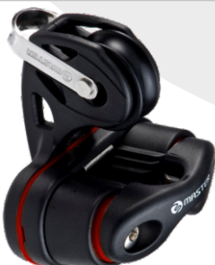
BB-2210F Single Cleat Lina: 6mm SWL : 100 kgs MAX: 390 kgs Waga: 47 g
